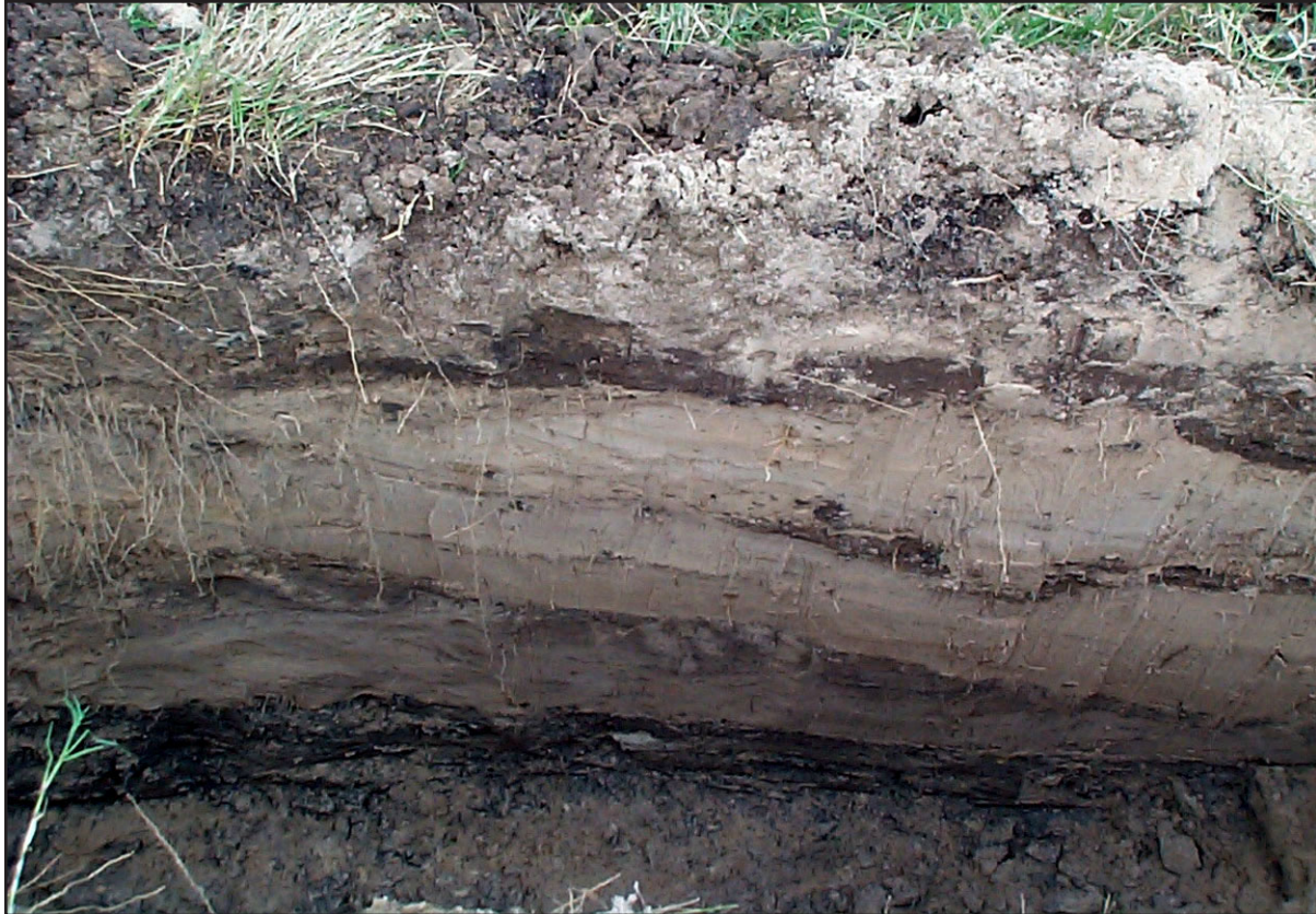
Figure 3-7. Profile of the south wall of BHT 14. Note laminated layers of clay and sand spoil deposit.
