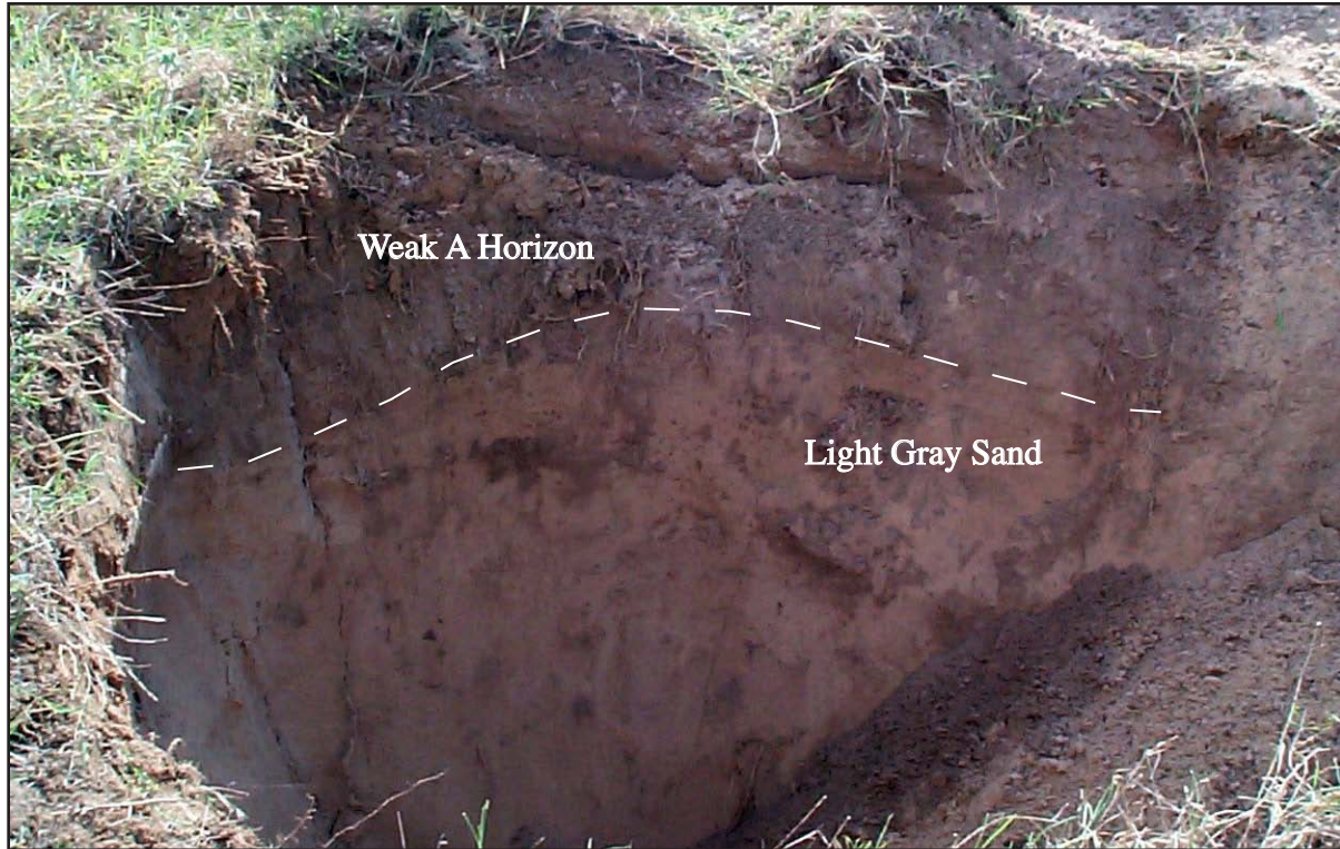
Figure 3-3. South wall of Backhoe Trench (BHT) 6 showing brown weakly developed sandy A horizon on top of light gray sand.
